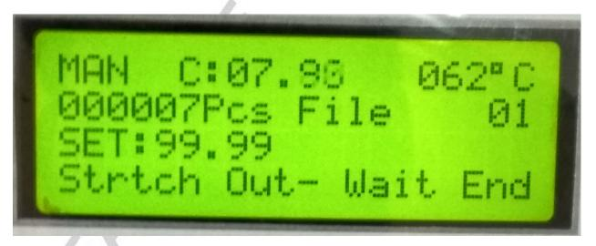
At main page, in first line there will be the current mode of machine. If machine will be in manual mode, it will display MAN, and if machine will be in auto mode it will display AUTO. Than after it will display the cycle time and current temperature.
