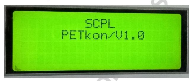
At power on, there is a name of the plc as well as the current programmed version will be display on screen.
