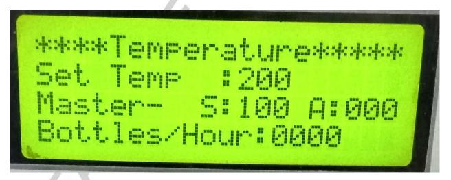
At temperature page, in second line it will display the set temperature. In third line it will display the master output value. Set value as well as actual value. In fourth line it will display the total estimated value of production of bottles per hour.
