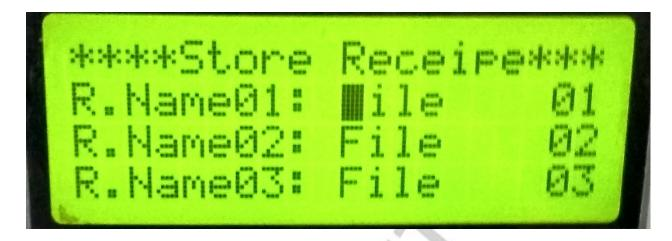
At store recipe page, it will display the name of all recipes as well as you can change the name of recipe by using numeric keys. To store the value of recipe, first of all select the recipe at by using page up/down key. And then press SELECT key to store the recipe.
